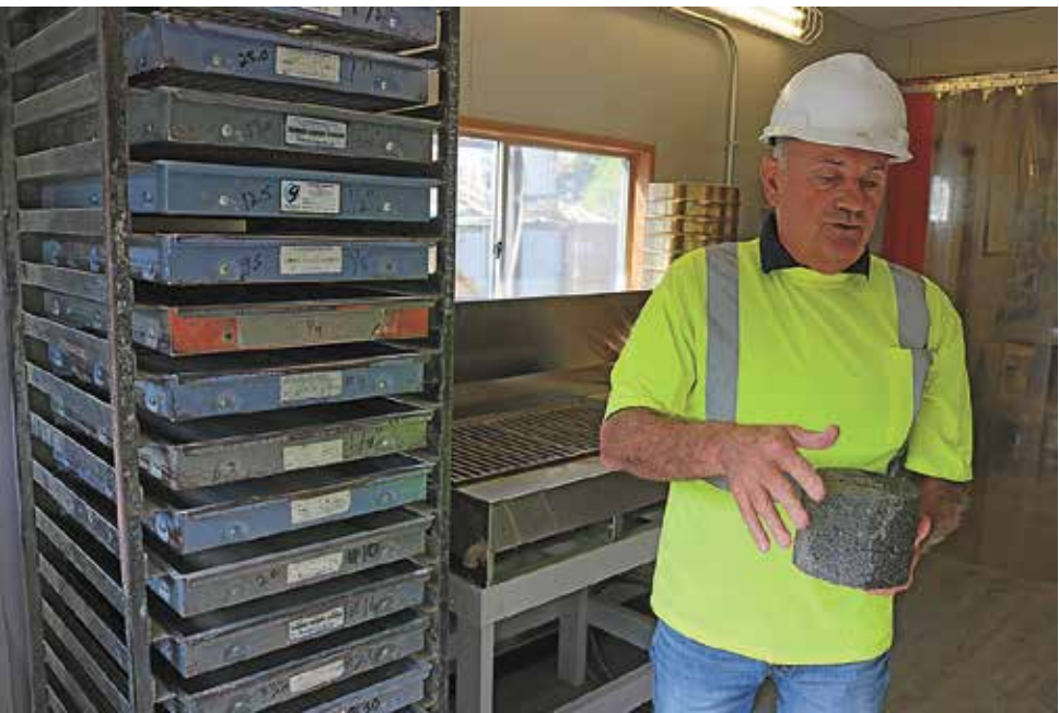
John Amato of Thalle Industries holds a core removed from newly laid asphalt to test its durability. The quarry, located on Route 9 in Fishkill, provides much of the asphalt and crushed stone used to build or repair local roads.
